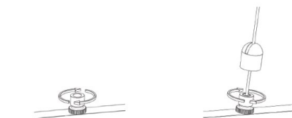
Dome Nut Installation
